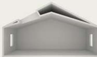
Although similar to a cathedral ceiling, vaulted ceilings feature a single sloping side or arched slope. This style may require a light shaft to be created between your ceiling and roof for the skylight.
