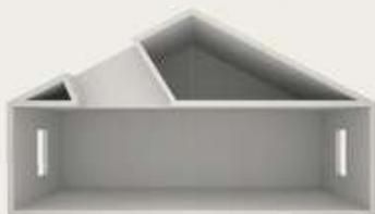
If you have flat ceilings, once your skylight is set outside, your installer will construct a drywall light shaft inside. This shaft directs daylight to the room below while hiding the attic space between your ceiling and roof.
